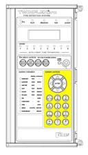
A context-driven highlighted-selection menu system is used to pilot around the menu system, automatically prompting you with the relevant options for your Access Level and system status.
